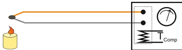
$$T_{\text{mes}} = \frac{V_{\text{mes}}}{\alpha(T)} + T_{\text{Comp}}$$
