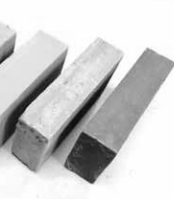
The unfired clay bricks tested
