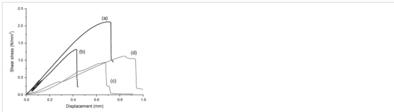
Fig. 4. Shear stress as a function of displacement for (a) SB2, (b) SB1, (c) HB2-90% and (d) HB2-40% samples.
