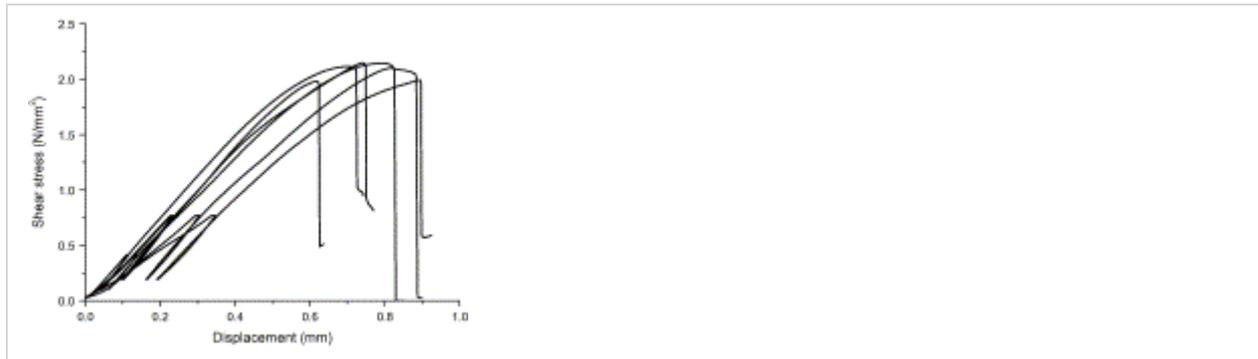
Fig. 3. Various values of shear stress as a function of displacement for the SB2 sample.
